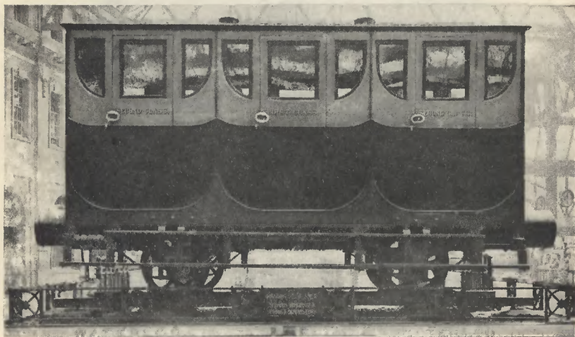
FIG. 6.— London and South Western Railway. Original Coach and Permanent Way used on the Bodmin and Wadebridge Branch from 1834 to 1886.
