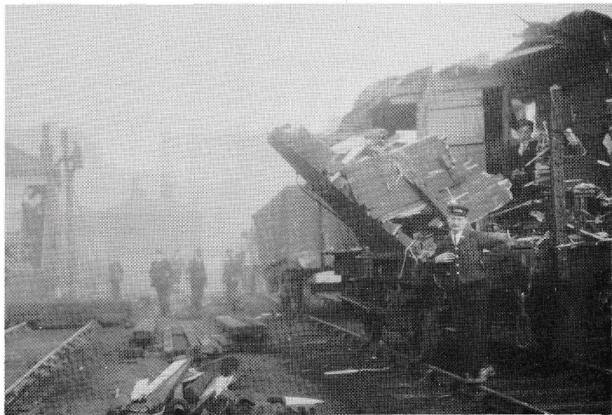
The end of a break van in a smash at Lockwood 28th October 1913. The vehicle is an early type with the cross-shaped break hanger but has tie rods to brace the 'W' irons of the under-frame .... a feature not seen elsewhere. All other details agree with Drg. 2309 of 1890.
