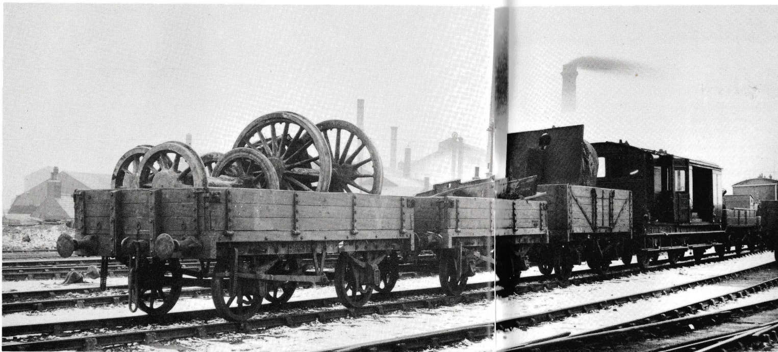
The wagons contain manageable pieces of the cut-up locomotive. The nearest wagon carries the two sets of carrying-wheels and the rear drivers while the second wagon has the left-hand water tanks. Both wagons are 3-plank dropside 10-ton types to Diagram 15 (numbers 7300 and 24641 respectively). The third wagon contains the firebox and part of the bunker water tank. This is a Diagram 16A 5-plank wagon which was a development from the earlier but similar 4-plank type built to Diagram 16. The tool van of the breakdown train stands in the background. Photograph taken 22 February 1916 at Penistone.
