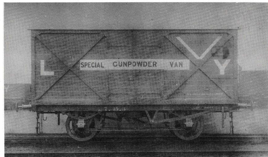
Diagram 95 Picric Acid Van as newly turned out in January 1917. Screw couplings and vacuum brakes are a necessary complement to such vehicles.
