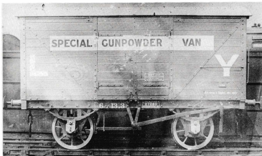
Van No.27289 of 1908 seen here in August 1914 and lettered "To be Returned to Maghull when Empty". In view of the dangerous contents, the three-link couplings and single brake-shoe each side seem inappropriate. The van is part of Diagram 60 but appears to be little different from the common Diagram 3 type.
