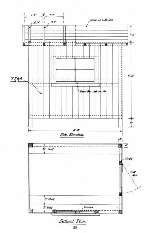
Scale 10 mm = 1 foot B.C.L 10.9984 7"×14" 0.0 0 0 Rim lock with 2 keys 3"x 3"4" - Strong Thinges 6"x14" Batters Section 6:0" Through Window End Elevation
