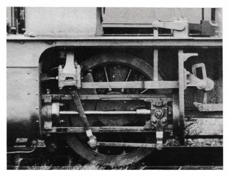
A close-up view of the Walschaert valve gear which should help all modellers faced with this feature. The view shows the balance weights on the driving wheel clearly and such small details as the steps up the back of the motion bracket.
