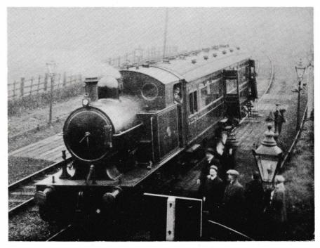
One of the first series (Nos. 3-8) of the railmotors pauses at Poulton Curve Halt with a Fleetwood to Blackpool (North) service about 1913. The locomotive cannot be identified but is in original condition. Several of the engine units were never altered apart from the chimney until the LMS period. The carriage has been altered and has received the lower type of gas lamps giving us the anomaly of an unaltered engine and a final condition carriage!
