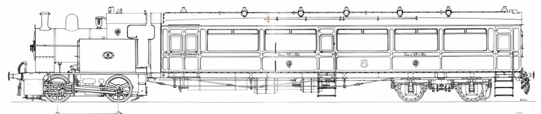
THE GAS CYLINDERS 1'-11" diam, x 7'-9%" long ARE HERE SHOWN DOTTED TO REVEAL THE DETAILS OF THE TRUSS RODS, QUEEN POSTS & TURN BUCKLES.
