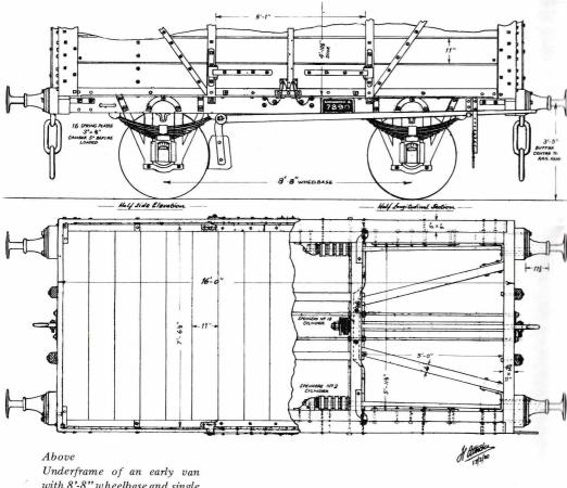
Underframe of an early van with 8'-8" wheelbase and single wooden brake block. The source for this drawing is a Newton Heath original signed by Attock and dated 17.2.1880 which is unsuitable for reproduction. India Rubber springs for buffers and drawbar, Attocks grease axleboxes and buffers mounted on shaped blocks of timber.
