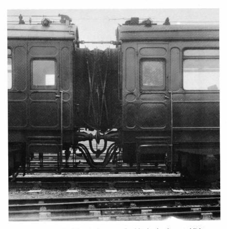
Trailer carriage on the left and railmotor on the right showing the control linkage over the corridor connection. Notice the wire which works the whistle and the slotted buffers. The pipes between the vehicles are the vacuum brake, steam heating and two for working the folding steps—one for each side.
