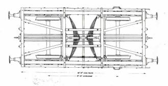
Later arrangement after adoption of 9'-0" wheelbase. Central leaf springs have replaced the rubber springs. Brakegear on one side only has a second lever on the other side, giving both levers at the same end of the vehicle.
