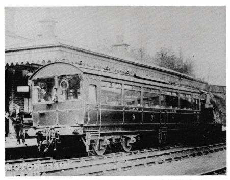
The carriage end of the first Horwich railmotor in original condition. The picture must have been taken in the first few years of service as the roof-boards are in the very high position adopted at the first. The circular device on the driver's window is a marine-type window wiper. The original type of bogie and the 'slotted' 4-bolt buffers are well shown in this view.
