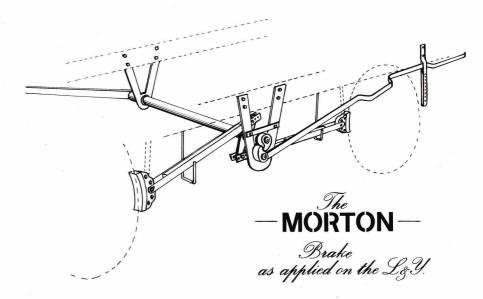
A few years prior to the opening of Newton Heath C & W works (c.1873), it became accepted practice to fit stock with Either side brakes (ESB), but both brake levers were at one end of the wagon—this both simplified the operation of the brakes and of course cheapened the cost.
