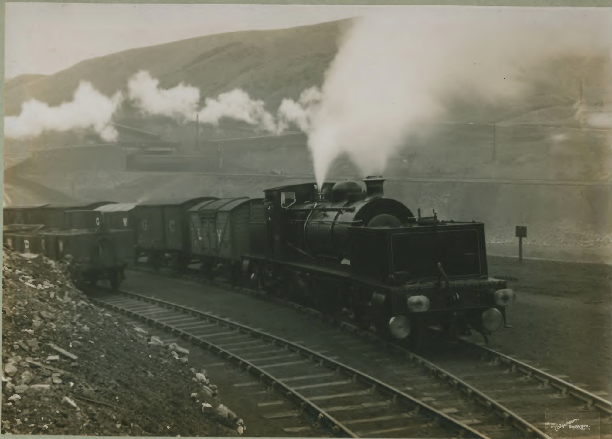
" GARRATT " ARTICULATED LOCOMOTIVE ascending 1 in 20 grade and about to negotiate 90 ft. radius curve, hauling 140 tons 8 cwt.
