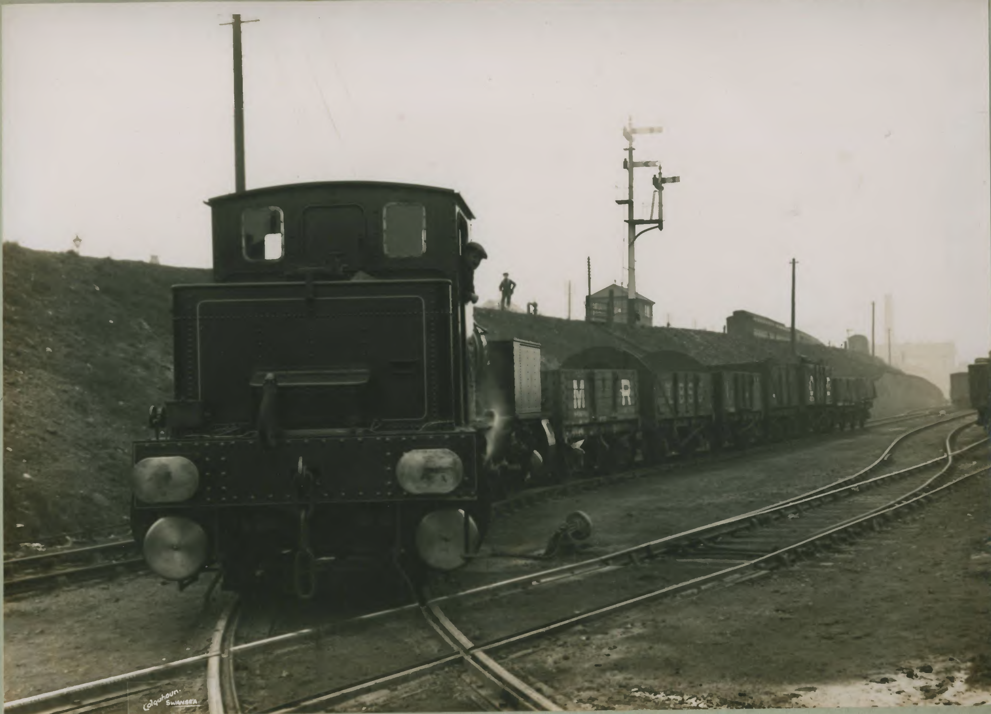
“ GARRATT ” ARTICULATED LOCOMOTIVE leaving Great Western Railway sidings and negotiating 97 ft. radius curve prior to descending 1 in 20 grade. The three distinct parts of the “ Garratt ” engine, which make up its flexibility can be distinctly seen in this photograph by following one’s eye along the running board.
