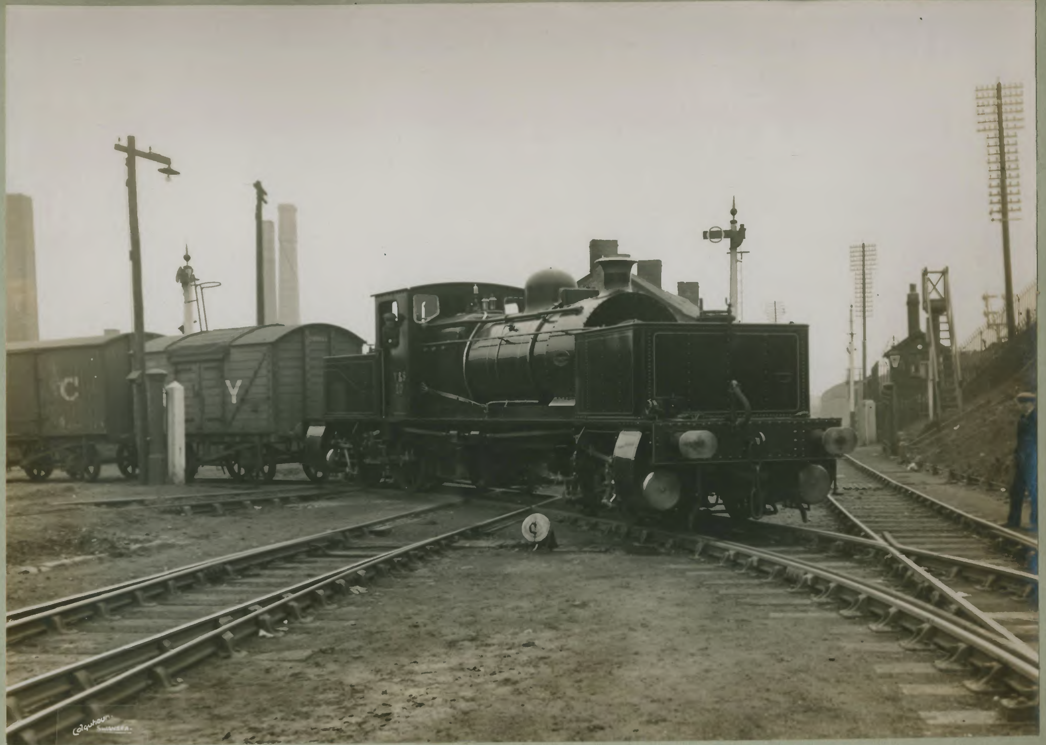
“GARRATT” ARTICULATED LOCOMOTIVE negotiating 97 ft. radius curve. This curve, as is seen, crosses the rails of the Great Western Railway and is, therefore, without super elevation.
